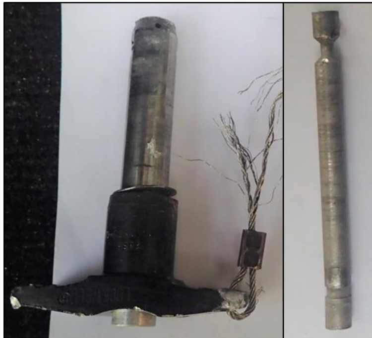
Photo No. 4: Torque Link Release Pin with Damaged Lanyard (Left) and Internal Retention Pin (Right)
