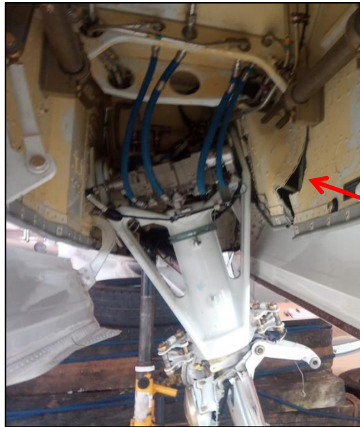
Photo No. 3: Damage to Aircraft Nose Structure
